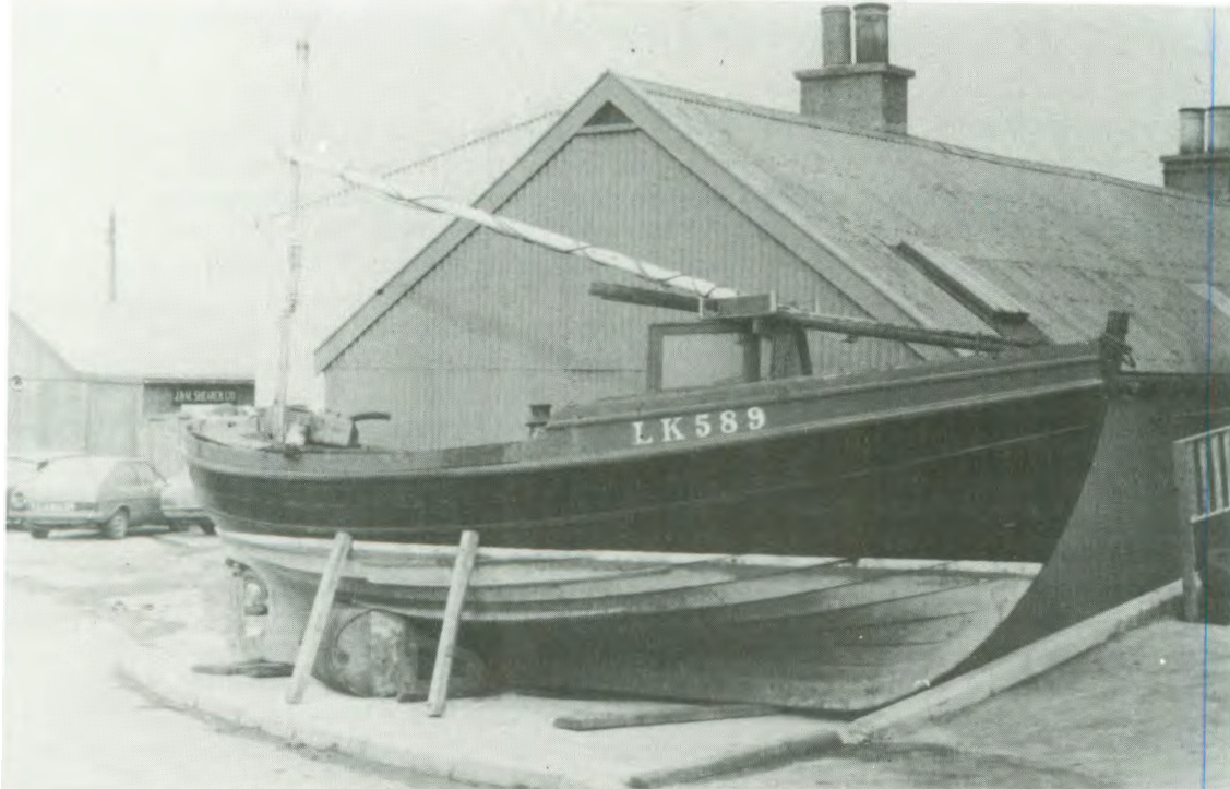
Figs. 8.3; 8.4.— Bow and stern three-quarter views of the UTILISE, LK 589. This is a fine example of the purpose-built motor craft built by Walter and Phillip Duncan for the inshore fishery during recent years. The lines of hull and planking, the functionalism of layout and fittings, epitomise attitudes and skills that represent the best of the ongoing Scandinavian tradition in Shetland. (Photographs: A.G. Osler)
