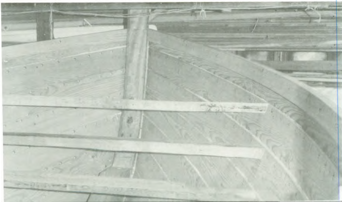
Figs. 8.5; 8.6. — Views of the exterior and interior of a 18 ft. pleasure/fishing craft under construction by Walter and Phillip Duncan, 1975. The larch wood shell planking is complete and the interior frames are being inserted, although temporary braces inside still help hold the shape fore and aft. The whole structure has been built with no physical 'memory aids' other than the occasional use of a simple midships check-mould, and a stem pattern used for an earlier boat. (Photographs: A.G. Osler)
