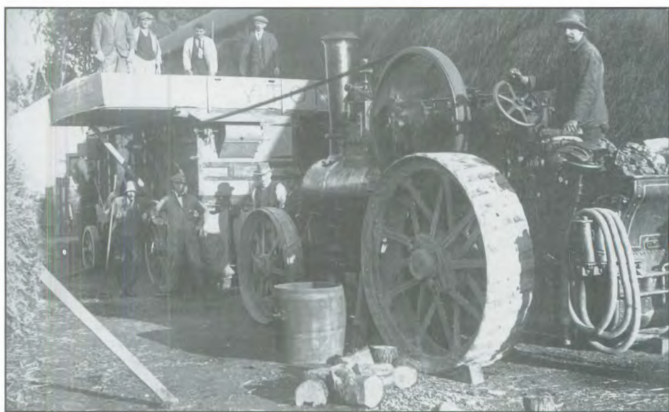
Figure 9: Threshing by steam at Ballamona farm, October 1941, using a Clayton and Shuttleworth 7 h.p. traction engine to drive a Clayton 54 inch threshing mill.
